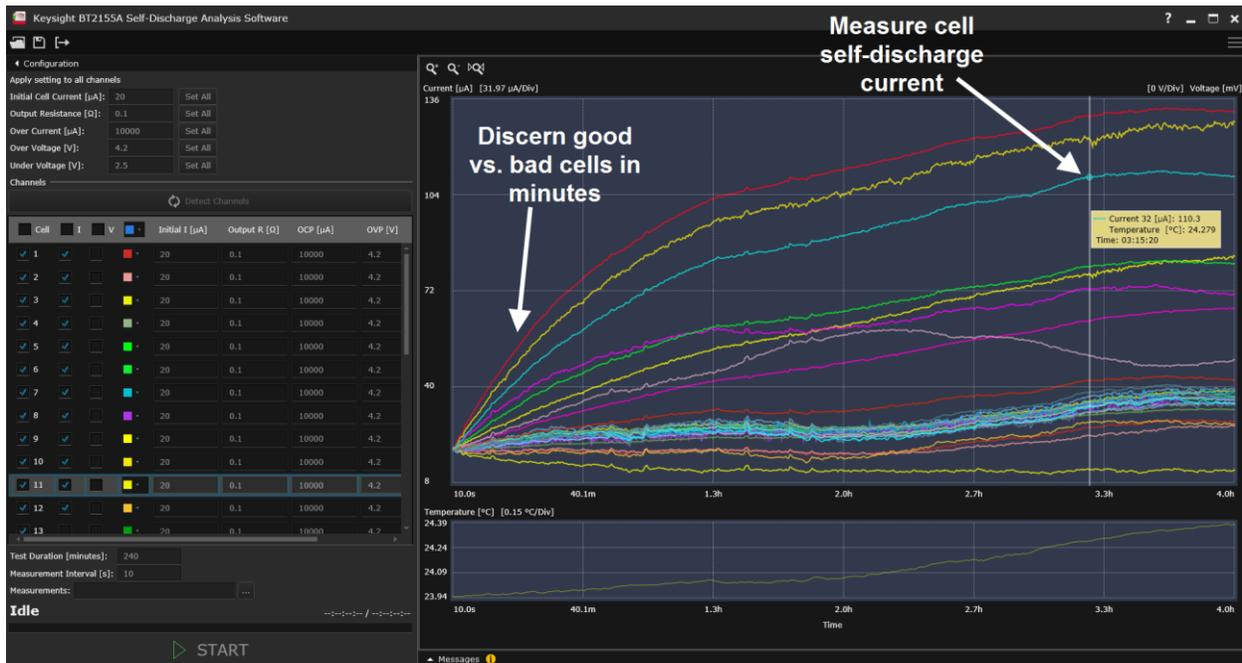
Figure 4. Results from 4-hour test of 18650 cells
